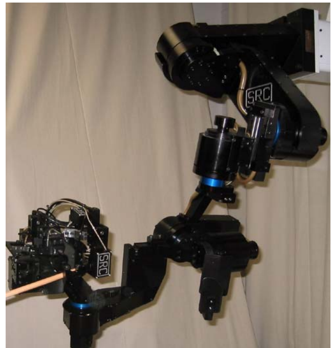
Fig. 2 Sarcos Master Arm robot, as used for the evaluations on our experiments
