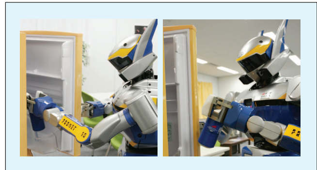
Figure 1. Work at AIST with the HRP-2 humanoid has combined high-level teleoperation with autonomous perception and control. This work has enabled a user to reliably control a complex humanoid robot to perform sophisticated manipulation tasks, such as retrieving a drink from a refrigerator [3].
