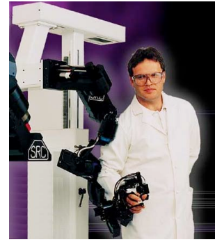
Fig. 1. 7 degree-of-freedom hydraulic robot: Sarcos Master Arm
