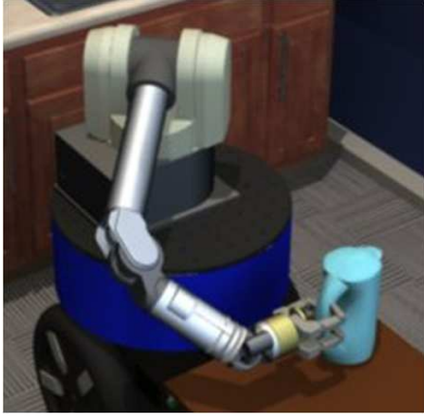
Fig. 2. The grasping posture at the time of object lifting from the surface depends on the object pose. Even for a 1-DoF change of object orientation, the allowable manipulator configurations can change significantly due to the different end-effector poses required to reach the object handle.
