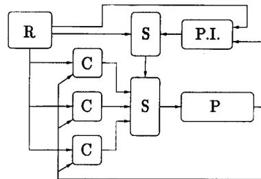
Fig. 1 A hybrid control system, R-reference generator, C-controller, S-scheduler, S-switch, P-plant, P.I.-performance index
