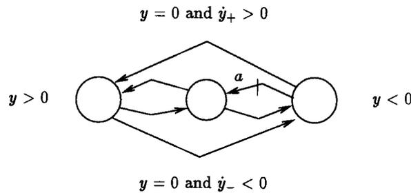
Fig. 4 System with one induced mode. Only one induced transition is indicated,  $a : (y = 0 \text{ and } \dot{y}_+ < 0)$
