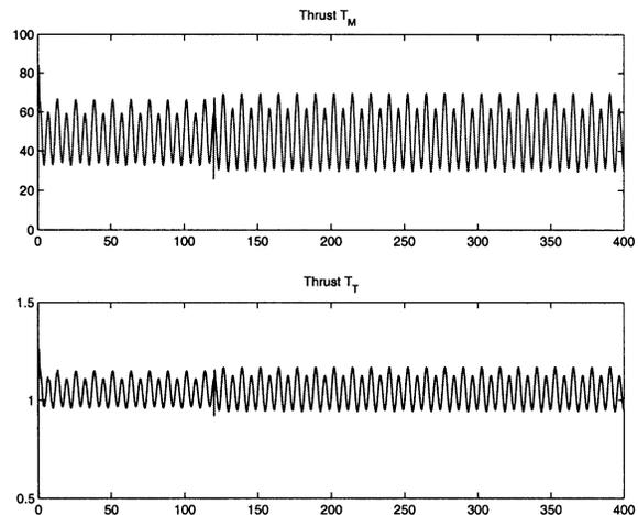
Fig. 9. Main rotor and tail rotor thrusts  $T_M(t), T_T(t)[N]$ .
